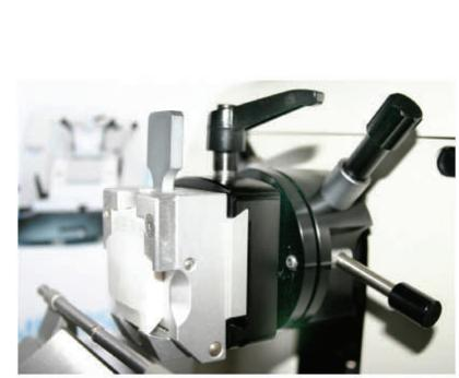
Precise orientation mechanism makes easy to adjust the specimen to the right position on the x/y axis
